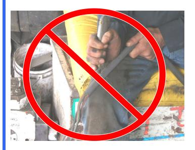
NEVER use any part of your body as a work surface to hold or support the object being cut.
