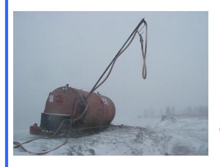
Install fuel stations that limit, the need for operators to climb and carry fuel nozzles and hoses.
